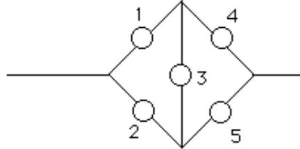
FIGURE 1. Representation of a simple bridge system
